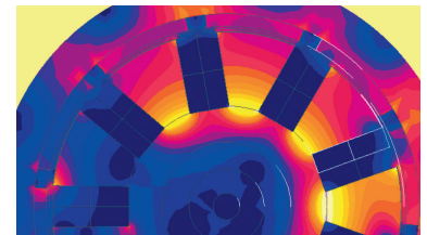
TOP: 2D Magnetic flux isovalues in the trapezoid Stator RFPM motor BOTTOM: 2D Magnetic flux density in the trapezoid Stator RFPM motor
